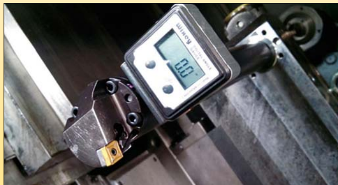
Figure 4: Aligning the boring bar
